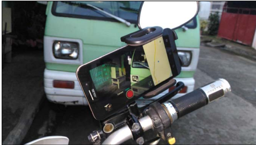
Figure 2.2-2 Mobile and Metal Holder Set-up fastened on a motorcycle (Routeshoot App running)
