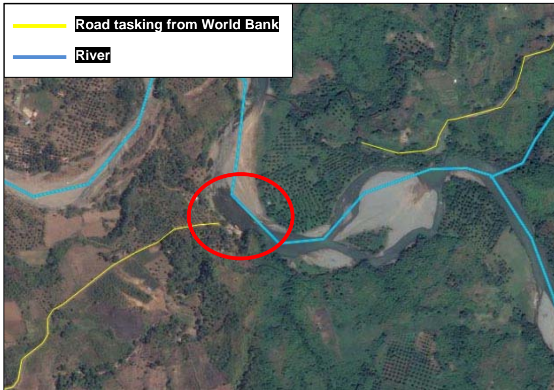
Figure 3.2.2-2 Road Tasking Cut by a River in Pange, Siayan
